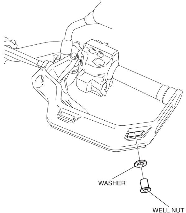
3. Install the left knuckle guard B as shown.
